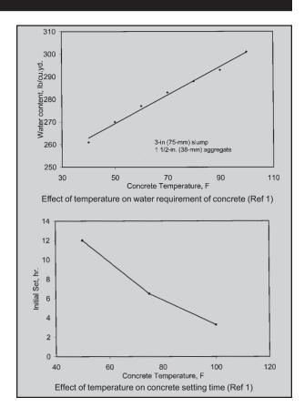
lowed by a cool night. High temperature also accelerates cement hydration and contributes to the potential for thermal cracking in massive concrete structures.
